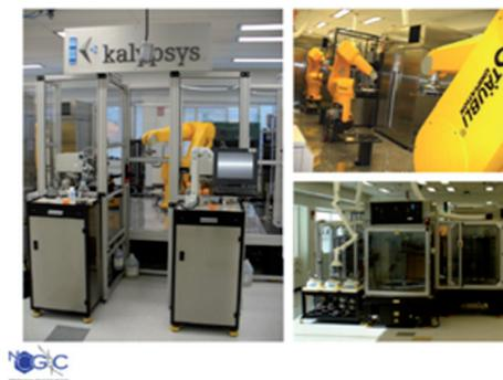
Yasgar A, Klumpp C, Hughes, et al. Kalypsys high-throughput robotic screening system: Making highly-efficient screening in 1536-well format possible. [www.wakousa.com](http://www.wakousa.com)
